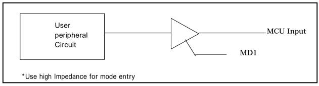
Fig. 3.3: Collision Prevention Circuit Using Three State Buffer
