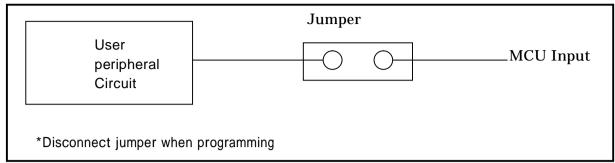
Fig. 3.2: Collision Prevention Circuit Using Jumper
